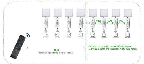
Range of control on 2.4G Smart system is not limited from the range of remote controller. In a large premises, exceeding the range of remote controller, drivers/dimers transmits signal among themselves and inspect the light state for each other. This is possible when distance between drivers/dimers is less than 10 meters.
